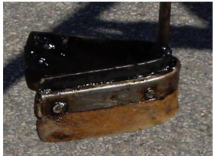
*Figure 9. Rubber Finishing Squeegee for Use with Cold Pour Sealant*
