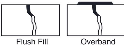
*Figure 6. Crack Sealing Common Configurations*
